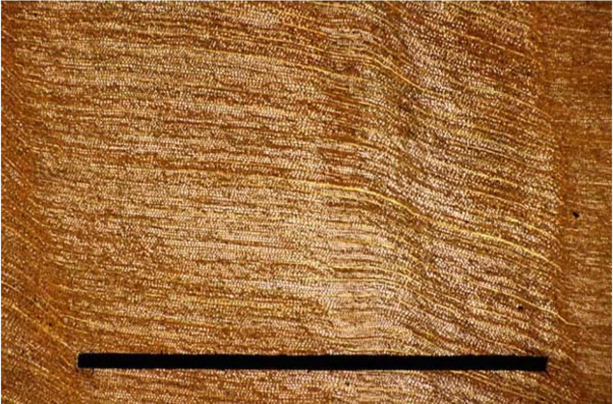
Figure 7. Cross section of wood from the stump shown in Figure 6. Note the lack of well- defined growth rings and “late or summer” wood. The bar scale indicates the amount of wood produced in one growing season.
